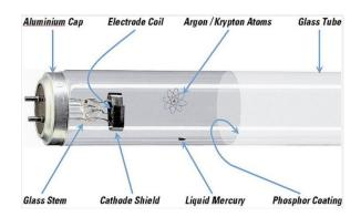
The advantages of fluorescent lights include energy-efficiency and producing light on the white end of the color temperature spectrum—which is desirable in some environments. Fluorescent lamps are also long-
