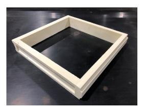
2. Hard rail is cut to size and used to construct the panel perimeter frame much like a "picture frame".
