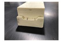
1. Hard rail is produced by injecting a 2-part structural foam mixture into metal molds. When the 2-parts of the foam mixture combine they chemically react to expand and fill the mold forming a solid structural foam. At Arctic we call them foam 2" x 4"s. Unlike a traditional wood 2" x 4", the strength of our foam 2" x 4"s is consistent throughout and they are not susceptible to mold, mildew, and rot.
