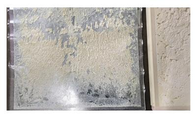
The chemical reaction of the foam while in contact with the hardrail and metal provides an extremely tight bond – so tight that the foam separates from itself while adhering to the metal when tested as part of our quality control process.
