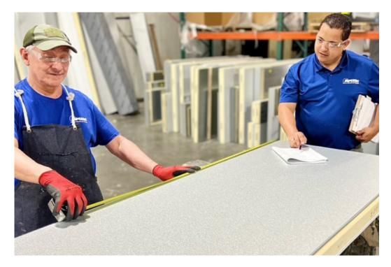
The panel is removed from the press and inspected prior to assembling your new walk-in.
