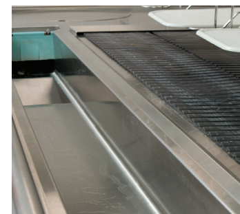
Built-in trough for scraps minimizes floor space
