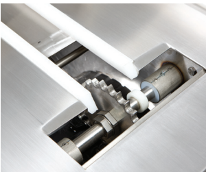
Sealed bearings require no lubrication
