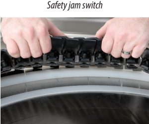
Slanted rollers allow easy removal of the belt at turns
