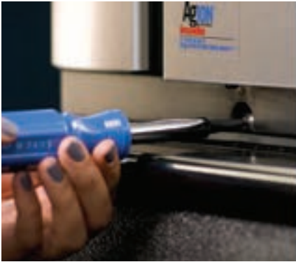
Loosen the two screws on the bottom of the front panel.
