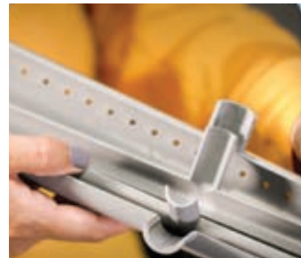
Completely disassemble the distribution tube.
