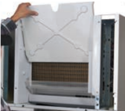
Remove the evaporator splash plate.
