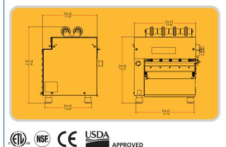
**Rollers:** 3.5" (8.89 cm) dia. 11" (28 cm) length **Scrapers:** Synthetic, spring loaded, Removable
